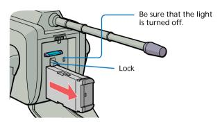
4 Install a fully charged battery pack arrow-wise. Be sure to install the battery pack until it clicks.
